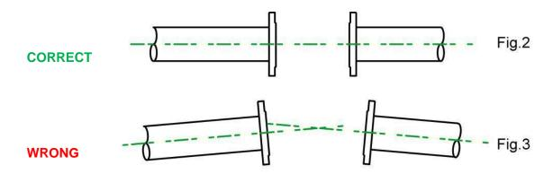
7- Make sure the pipe flanges are perfectly parallel (Fig. 2) and not inclined (Fig. 4); this would cause the same drawbacks listed in the previous point.
