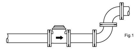
5- When installing, be careful with the arrow indicating the flow of water placed on the body of the meter.
